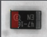
Capacitor Oriented Backwards
